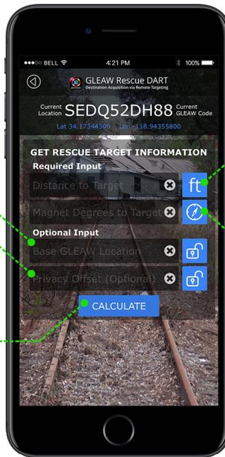
Distance to the target is input here. Touching the units icon switches between feet and meters.
